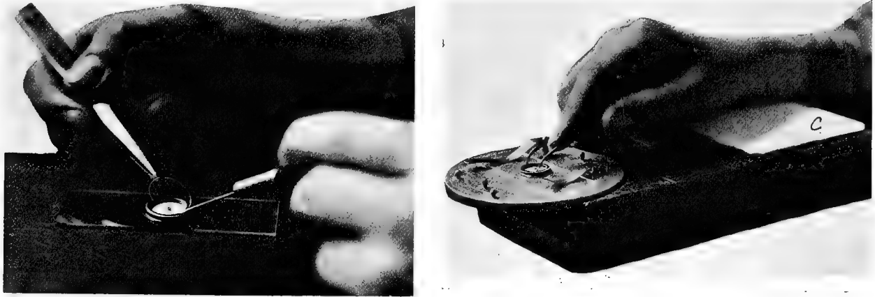
FIG. 21.—A. Method of placing cover slip on a fluid mount. B. Turntable in action and cover slip being pressed into position. C. Mounting plate on turntable carrier.
